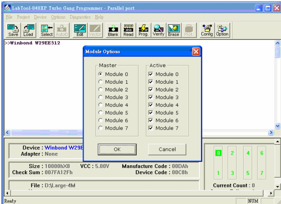
Figure 4-9 Master socket selection, active socket selection
