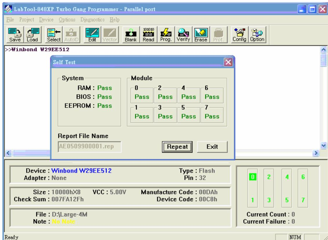
**Figure 4-13 System and all modules self test screen**
