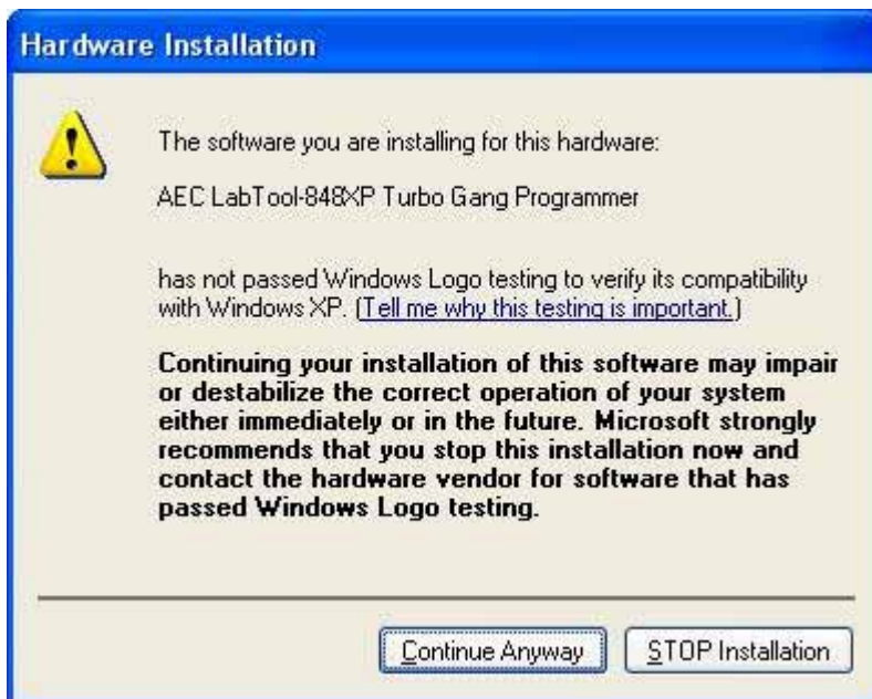
Fig6-4 : Press “ Continue Anyway” . If you select the other button, the O.S. will has a wrong “!USB Device” in your PC.
